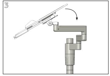
Rotate the Keyboard Platform back towards a flat position.
