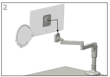
With the VESA bracket oriented "TOP" up, slide the bracket over the arm mount until it clicks into place.
