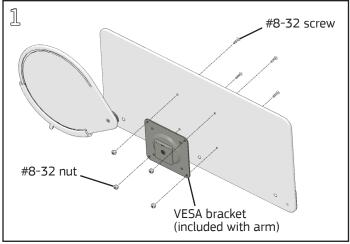
Align the VESA bracket (included with arm, order arm separately) with the holes near the center of the Keyboard Platform. Fasten bracket to platform with (4) #8-32 flat head screws and (4) #8-32 acorn nuts using a #2 Phillips screwdriver and 11/32" nut driver.
