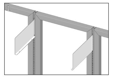
Engage the brackets in the left and right sides of the frame or frame span. Ensure the brackets are firmly seated in the hanger frame slots and use a **tape** measure to verify both the right- and left-hand brackets are at the same height.
