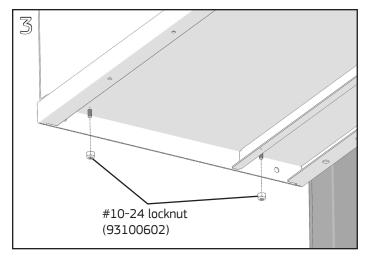
Hold the brackets down to prevent disengagement and fasten each end of the shelf with (2) #10-24 locknuts. Apply a torque of 20 in-lbs. to each nut with a %" socket and torque driver.
