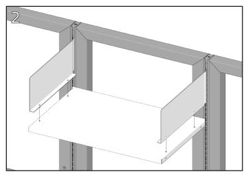
Align the holes in the top of the shelf with the threaded studs in the bottom of the brackets. The shelf lip can be oriented either towards the front or the back.
