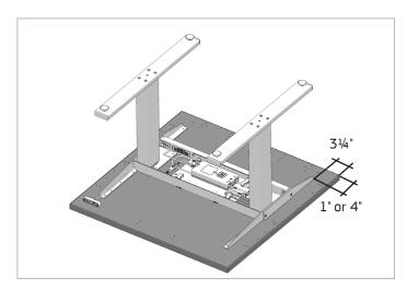
8. Install the top (not included) with base upside down. Center the base over the width and depth of the top rear overhang is 2" for a 24" or 30" deep top, or 5" for a 36" deep top. Drill 1/8" diameter x 1/2" deep pilot holes to align with the holes in the stretcher top supports as needed.
