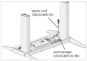
5. Attach the power cord to the port on the control box labeled "AC" and route the cord through the cord manager in the back corner of the stretcher.
