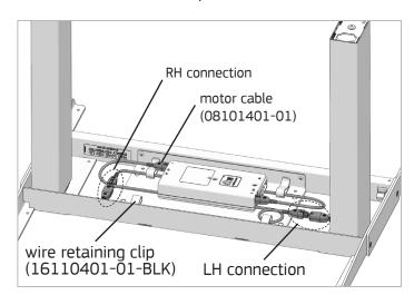
4. Flip unit upside down. Connect the leg cables to the motor cables that are preassembled to ports 1 and 2 of the control box. Manage excess cable length with wire retaining clips.
