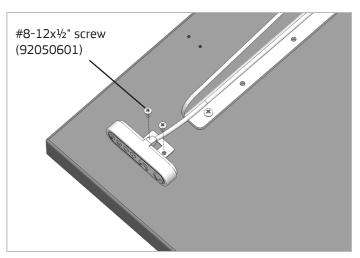
10. Secure the hand control with (2) #8-12x½" Phillips pan head screws.
