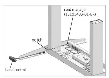
6. Route the end of the hand control cable through the front stretcher notch, along side the leg, and through the cord manager in the back corner of the stretcher. Plug the cable into the port labeled "A1".
