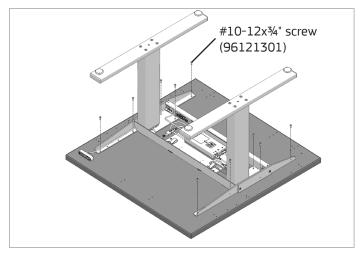
9. Attach top to the base with (5) #10-12x¾" Phillips pan head screws per side. Ensure one of the five screws on each side is installed in the back bracket hole.
