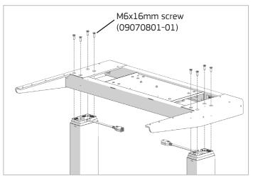
2. Place legs on the floor oriented with cables at top, space legs to match the width of the stretcher. Align countersunk holes in stretcher with tapped holes in the top of the legs. Install (4) M6x16mm socket flat head screws in each leg to secure the stretcher. Do not exceed a screw torque of 10 Nm (88.5 in.-lbs.).
