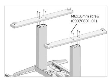
7. Attach each foot to the bottom of the leg with (4) M6x16mm socket flat head screws using a 4mm Allen wrench. Do not exceed a screw torque of 10 Nm (88.5 in-lbs.). If applicable, attach casters. Install casters with brakes at front of base.
