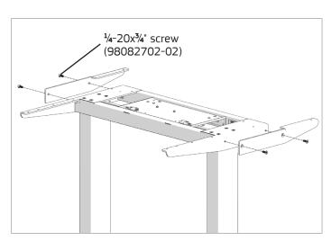
3. Fasten rear brackets to stretcher with (2) ¼-20x¾" Phillips flat head screws uing a **#2 Phillips bit and cordless drill**.
