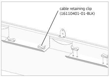
6. Install cable retaining clips in the double hole patterns in the bottom of the cable trays.
