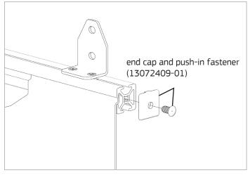
5. Fasten an end cap to each end of the rail with a push-in fastener.
