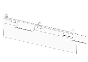
4. Slide the cable trays in the rail slot, centering tray between pass-thru notches in modesty panel.
