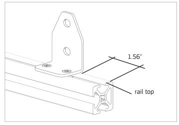
Slide the bracket sets into the top of the rail. For panels larger than 48", center one bracket set over the width of the rail and tighten with a #2 Phillips screwdriver. Position the remaining bracket sets 1.56" from each end of the rail and tighten securely.
