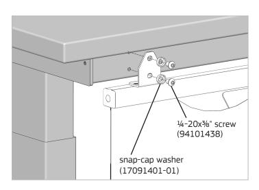
7. Align the rail brackets with the tapped holes in the back of the ErgoStat Pro stretcher. Fasten each bracket with (2) snap-cap washers and (2) ¼"-20x¾" socket button head screws, tighten securely with a 5/32" hex wrench.
