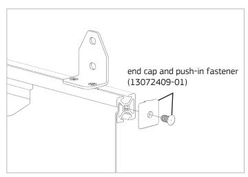
4. Fasten an end cap to each end of the rail with a push-in fastener.
