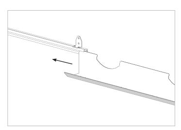
3. Slide the tray into the slot on the rail.
