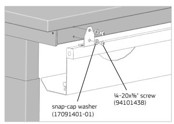
6. Align the rail brackets with the tapped holes in the back of the ErgoStat Pro stretcher. Fasten each bracket with (2) snap-cap washers and (2) ¼"-20x¾" socket button head screws, tighten securely with a 5/32\* hex wrench.
