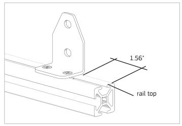
2. Slide the bracket sets into the top of the rail. For trays larger than 48", center one bracket set over the width of the rail and tighten with a **#2 Phillips screwdriver**. Position the remaining bracket sets 1.56" from each end of the rail and tighten securely.
