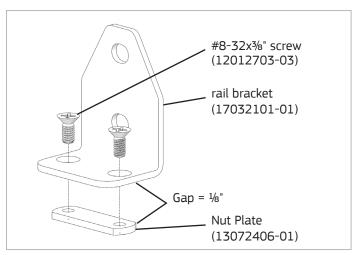
1. Preassemble a nut plate to each rail bracket using (2) #8-32x¾" Phillips flat head screws. Leave approximately a ⅓" gap between the bottom of the bracket and top of nut plate. Cable Trays that are 48" wide or less will require two bracket sets. Three bracket sets are required for trays wider than 48".
