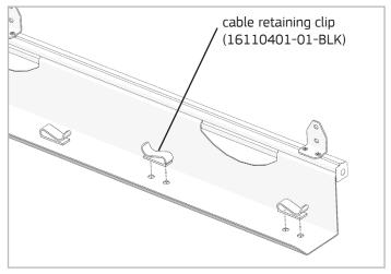
5. Install cable retaining clips in the double hole patterns in the bottom of the cable tray.
