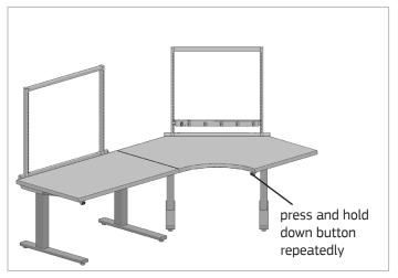
6. To properly initialize the synchronization of the bases, press and hold the down button on the control switch of either hand control until the bases come to a complete stop in the lowest position. Release the down button and wait 2-3 seconds. Then press the down button again.
