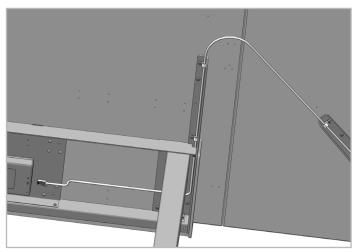
5. Continue routing the cable through the cable managers along the bracket of the adjacent ErgoStat Pro Base, through the front stretcher notch, and inside the stretcher of the adjacent base, plugging other end of the cable into port "A2" on the second base. Manage excess cable with stretcher cord managers.
