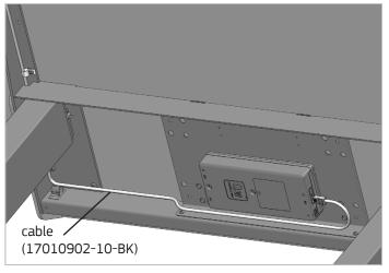
4. Connect 10' black cable to the port labeled "A2" on one of the bases. Route cable alongside the leg and through the front stretcher notch of the first base. Insert the cable in the cable manager locations.
