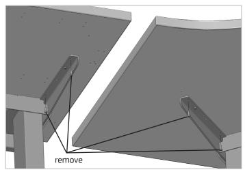
2. Remove the front screw and screw closest to the stretcher on the adjacent top support of each ErgoStat Pro Base using a #2 Phillips screwdriver.
