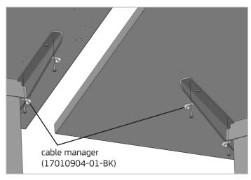
Reinstall each screw with a cable manager attached on each ErgoStat Pro Base.
