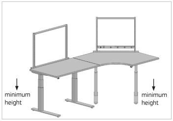
1. Assemble top surfaces to ErgoStat Pro Bases to be synchronized per installation instructions. Lower both bases to minimum height.
