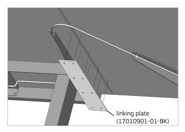
7. Align the top surfaces as desired. Use the linking plate to mark appropriate pilot locations at surface joint. If connecting rectangular tops, the front and back holes in the plate will align with an existing hole pattern and only four additional pilot holes will need to be added. Drill pilot holes using a 1/6" drill bit and cordless drill/driver.
