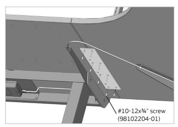
8. Attach the plate to the surfaces with (8) #10-12x<sup>3</sup>/<sub>4</sub>" Phillips flat head screws using a #2 Phillips screwdriver/bit.
