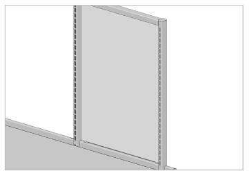
2. Slide insert up to the top flange of the Riser Panel and then press bottom of insert into the bottom of the panel. Ensure all magnets on the back of the insert are contacting the Riser Panel.
