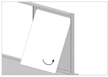
1. Center the width of the Tackable Insert between the flanges of the Riser Panel near the top.
