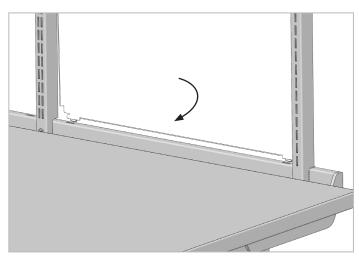
3. Rotate the bottom of the panel/board towards the bottom of riser frame, aligning the bottom tabs of the panel/board with the slots in the bottom tube of the riser frame.
