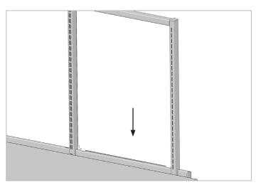
4. Allow the panel/board to drop into place, resting on the bottom tube of the riser frame.
