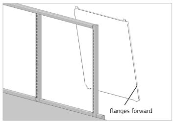
If installing panel/board with flanges forward, install board from rear of riser frame. If installing the panel/ board with flanges toward back of station, install board from front of riser frame.
