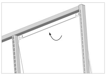
2. While holding panel/board at an angle, align the top tabs of the board with the slots on the underside of the top tube of the riser frame.
