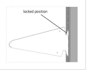
3. Rotate anti-dislodgement clip down until bottom of the clip snaps into the hole near the top hook of the shelf bracket. Repeat on opposite side.
