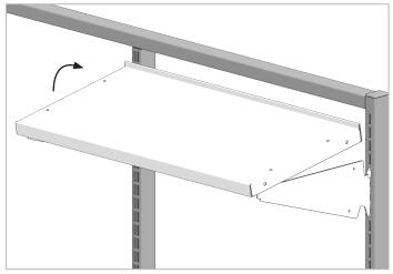
4. Align the front tips of the shelf brackets with the inside faces of the shelf sides. Rotate the shelf back until it drops over the back of the shelf brackets.
