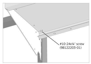
5. Install one #10-24x¼" Phillips pan head screw under the shelf near the back in the hole of each bracket. Fasten securely with a #2 Phillips screwdriver or bit with cordless drill on both sides of the shelf.
