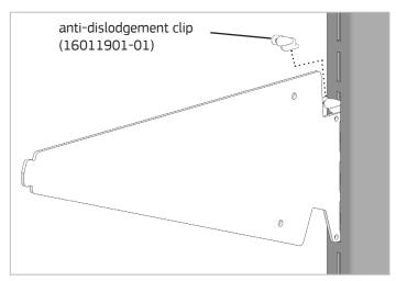
2. Insert tip of anti-dislodgement clip into slot above top hook of shelf bracket as shown.
