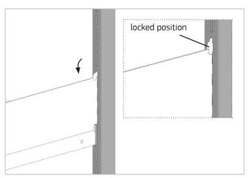
4. Rotate anti-dislodgement clip down until bottom of the clip snaps into the hole near the top hook of the shelf bracket. Repeat on opposite side.
