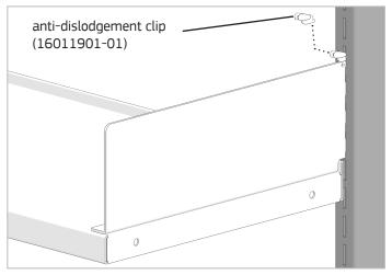
3. Insert tip of anti-dislodgement clip into slot above top hook of shelf bracket as shown.
