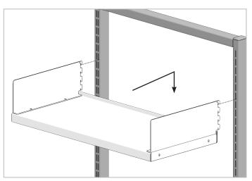
2. Insert bracket hooks into slots in ErgoStat Pro Riser Frame. Push shelf down to ensure it is firmly seated.
