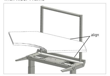
1. Attach Riser Frame to the base per instructions. Position the top on the base centered left to right with the back of the top aligned with the back of the stretcher.
