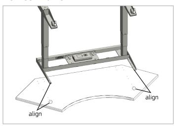
1. Flip the top upside down. Center the base over the width of the top, aligning the front pilot holes with the holes in the front of the top supports.
