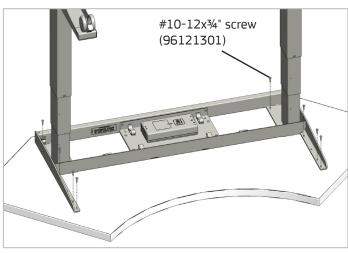
2. Attach the top to the base with (5) #10-12x¾" Phillips pan head screws per side. Secure the hand control with (2) #8-12x1/2" Phillips pan head screws.
