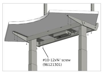
2. Attach the top to the base with (5) #10-12x<sup>3</sup>/<sub>4</sub>" Phillips pan head screws per side. Secure the hand control with (2) #8-12x<sup>1</sup>/<sub>2</sub>" Phillips pan head screws.
