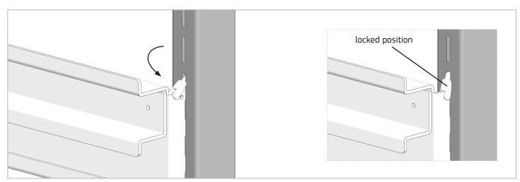
3. Rotate the anti-dislodgement clip down until bottom of the clip snaps into the hole near the top hook of the rail. Repeat on the opposite side.
