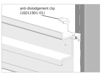
2. Insert tip of anti-dislodgement clip into slot above top hook of rail as shown.
