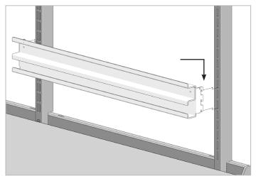
Align hooks in ends of ErgoStat Pro Slatwall/Bin Rail with slots in ErgoStat Pro Riser Frame. Insert hooks into slots and push down to ensure rail is firmly seated.
