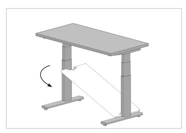
3. Hold shelf at an angle and insert between legs of base, centered notch on each side of shelf around leg. Rotate shelf down to flat position.
