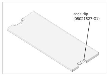
2. Install six (6) edge clips in notched area of shelf, three per side.
