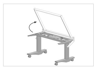
3. Rotate the Riser Frame back into its upright position.
