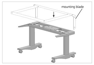
1. Center ErgoStat Pro Riser Frame over ErgoStat Pro Base with mounting blades outboard of base top supports. Rest riser face down on top of base.
