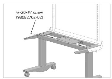
4. Install ¼-20x¾" Phillips flat head screws into the front mounting blade hole on each side of the Riser Frame. Tighten all four screws securely with a #2 Phillips screwdriver.
