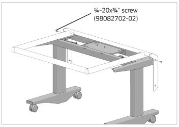
2. Align the rear holes in the riser mounting blades with the rear holes in the base top supports. Fasten with a ¼-20x¾" Phillips flat head screw using a #2 Phillips screwdriver.
