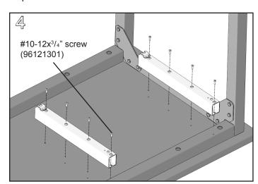
Mount the brackets to the surface with (4) #10-12x<sup>3</sup>/<sub>4</sub>" Phillips panhead screws per bracket using a **cordless drill** and **#2 Phillips bit**.
