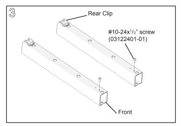
Preassemble one #10-24x<sup>1</sup>/<sub>2</sub>" Phillips truss head machine screw in the front tapped hole of each bracket, leaving a <sup>1</sup>/<sub>4</sub>" gap between the underside of the screw head and bracket.
