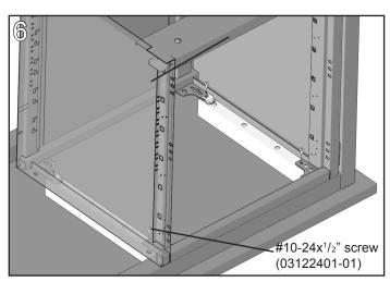
Tighten the front screw and install an additional  $#10-24x^1/2$ " screw at the front and back of the left and right sides of the cabinet. Securely tighten all screws.
