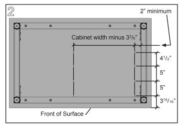
Mark hole locations for Cabinet Brackets as shown. Bracket may be used as template. Note cabinet will overhang hole pattern so ensure there is at least 2" clearance left and right of the hole pattern. Drill pilot holes with 1/8" **drill bit** and **cordless drill/driver**, 1/2" depth recommended.
