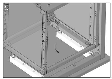
Remove doors, drawers and shelves from Suspended Base Cabinet. Align the centers of the keyslot holes in the front of the cabinet with the screws from step 3. Place cabinet against bracket and pull cabinet forward. The rear keyslot plates on the cabinet will catch under the rear clip of the bracket and the front screw will slide in the front keyslot.
