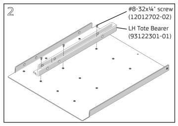
Lay the left-hand Tote Holder panel flat and assemble a left-hand tote bearer in all locations except the top with (3) #8-32x¼" Phillips flat head screws per bearer using a #2 Phillips screwdriver.
