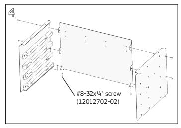
Assemble left and right Tote Holder panels to Tote Holder back using (6) #8-32x¼" Phillips flat head screws.
