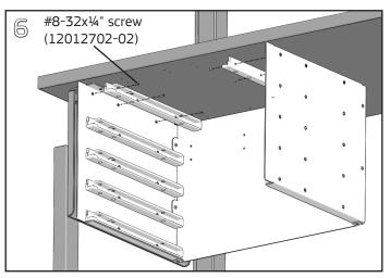
Attach the left and right tote bearers in the top locations of the side panels with (3) #8-32x¼" Phillips flat head screws per bearer using a #2 Phillips screwdriver.
