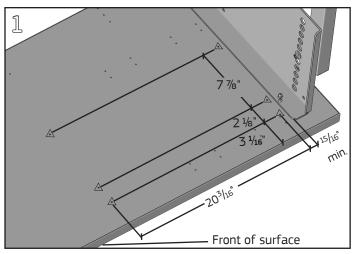
Determine placement of Tote Holder along width of surface. Mark and drill (6) ½" deep pilot holes in the surface per dimensions using a 1/8" Drill Bit and cordless drill/driver
