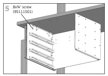
Align holes in top flanges of Tote Holder with the pilot holes in the surface. Attach with (6) #8x¾" Phillips flat head screws using a #2 Phillips driver.
