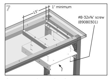
If mounting Auxiliary Work Surface to Storage Accessory Mounting Brackets on a 4-Legged Table, attach Storage Accessory Mounting Brackets with a 13" spacing and fasten Auxiliary Work Surface housing to the brackets with (4) #8-32x3/8" Phillips pan head screws in the outboard pattern of keyslots in the Auxiliary Work Surface housing.
