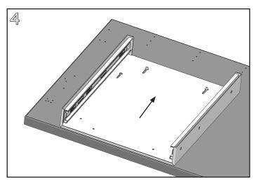
Align the inboard pattern of keyslots in the Auxiliary Work Surface housing with the attachment screws and slide the housing back.
