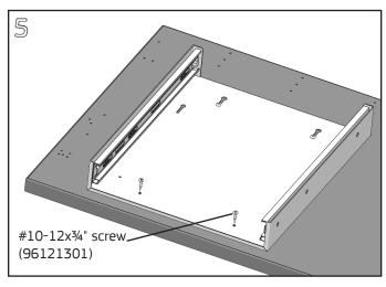
Install (2) additional #10-12x¾" Phillips pan head screws near the front of the housing. Tighten all (4) screws securely.
