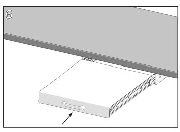
Align the slide members attached to the Auxiliary Work Surface with the slide members in the housing and push the surface into the housing until slides are fully engaged.
