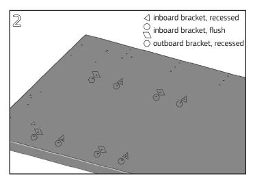
Determine the left-right mounting position for the Auxiliary Work Surface based on the location of the top supporting bracket. The surface can also be positioned flush or recessed relative to the front edge of the top.
