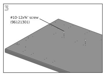
Install (2) #10-12x¾" Phillips pan head screws in the rear hole locations. Do not tighten fully; leave a ½" gap between the underside of the screw and top.
