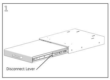
Remove the work surface from the housing by fully extending the slides and pressing the disconnect lever on the side of each slide.
