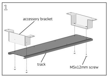
Attach accessory brackets to the front and back of the computer accessory track with (2) M5x12mm socket drive screws per bracket using a **3mm Allen wrench**.
