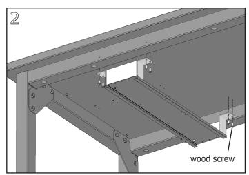
Fasten accessory brackets to the bottom of the surface behind front rail of table with (8) of the wood screws provided with the computer accessory using a **cordless drill** and **#2 Phillips bit**. Ensure proper clearance for the width of the computer accessory when attaching brackets.
