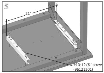
Orient brackets with the arrow end pointing towards the front of the table. Space the brackets 21" apart. Attach brackets to the surface with (6) #10-12x3/4" screws using a #2 Phillips bit and cordless drill.
