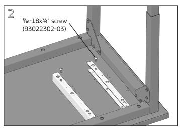
Insert (2) 16-18x3/4" Phillips pan head screws in the back weldnuts of the brackets, leaving a 1/4" gap between the underside of screw head and bracket.
