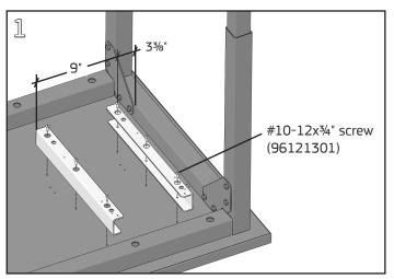
Orient brackets with the arrow end pointing towards the front of table. Space brackets 9" apart and allow clearance under table for the 15" wide pedestal. For a close fit of the pedestal on the left/right side of the table, position bracket approximately 3%" from the inside of the table leg. Attach brackets to surface with (6) #10-12x¾" screws using a #2 Phillips bit and cordless drill.
