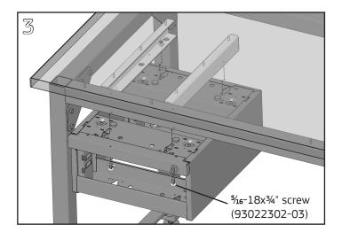
Remove pedestal drawers per installation instructions. Align center of rear keyslots in pedestal with the preinstalled screws in the brackets. Slide the pedestal back to engage screw. While supporting the front of the pedestal, install (2) \$\frac{5}{16}-18x^3/4\frac{3}{4}\frac{3}{4}\frac{1}{4}\$ Phillips pan head screws through the front keyslots of the pedestal in the front weldnuts of the brackets. Tighten all four screws with a **#4 Phillips screwdriver**.
