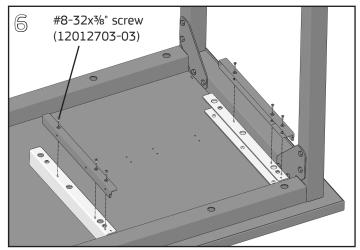
Align holes in the top of the tote/drawer bearers with the tapped holes in the brackets. Fasten bearers to the brackets with (3) #8-32x3/8" Phillips flat head screws per side.
