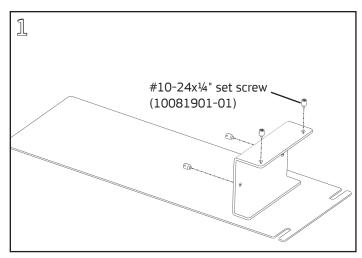
Preassemble (4) #10-24x¼" set screws in the tapped holes on the side and back of the bracket. If desired, predrill mounting holes in the bracket face for the component to be mounted to the bracket (components and component mounting hardware not provided).
