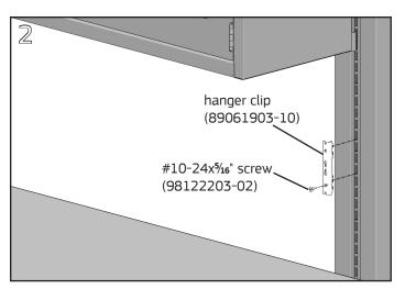
Install hanger clip on the left or right side of the frame. Install a  $\#10-24x\%_{16}$ " Phillips pan head screw into the bottom hole of the clip. Leave a %" gap between the screw and clip.
