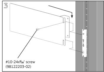
Place the bracket assembly around the vertical tube of the frame, align the lower slot in the bracket with the screw in the hanger clip and slide down. Install a #10-24x516" Phillips pan head screw into the top hole of the clip and fully tighten both screws with a #2 Phillips screwdriver.
