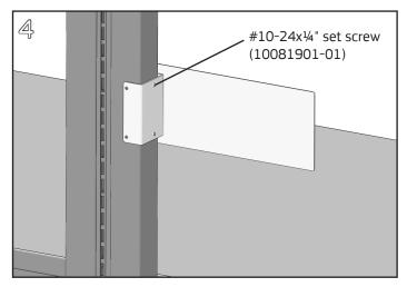
Fully tighten all set screws on the side and back of the bracket with a 3/32" Allen wrench.
