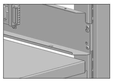
If necessary, remove electrical distributor face cover.
