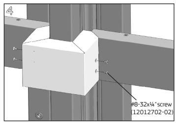
Align the countersunk holes in the cover with the tapped holes in the bracket flanges. Fasten the cover with two #8-32x¼" Phillips flathead screws on each bracket using a #2 Phillips screwdriver.
