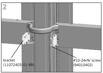
Attach a bracket to each distributor end with two #10-24x%" Phillips pan head screws, fastening into the two tapped holes in the clip of the Electrical Distributor. Tighten screws with a #2 Phillips screwdriver.
