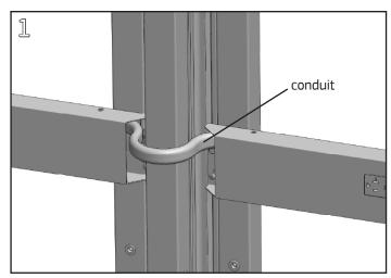
Install Electrical Distributors and Jumper Cable per individual product installation instructions. Route the Entry Cable conduit near the top of the Electrical Distributor.
