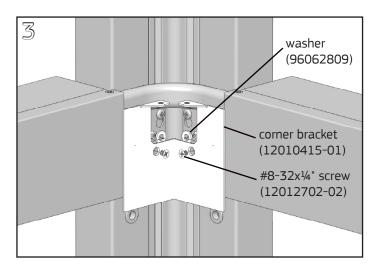
Align the countersunk holes in the corner bracket with the standoffs attached to Electrical Distributors. Insert a #8-32x¼" Phillips flathead screw through each counter-sunk hole, then a nylon washer, and tighten screws with a #2 Phillips screwdriver.
