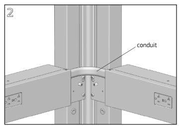
Install Electrical Distributors and Jumper Cable per individual product installation instructions. Route the Jumper Cable conduit above the Electrical Distributor hanger clips.
