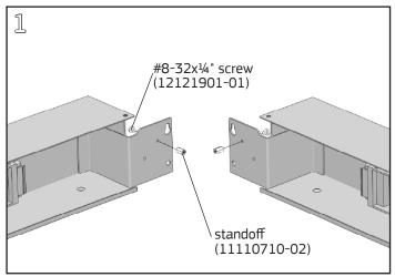
Before installing the Electrical Distributors on the frames, install a #8-32x¼" Phillips panhead screw in the upper tapped hole on the distributor base end near the corner connection. Fasten a hex standoff to the end of each screw and tighten with a ¼" wrench and #2 Phillips screwdriver.
