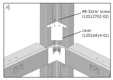
Place the cover on top of the support tabs of the corner bracket. Install a #8-32x¼" Phillips flathead screw through each countersunk cover hole and tighten with a #2 Phillips screwdriver.
