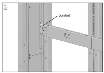
Install Vertical Distributor, Electrical Distributor and Entry Cable per individual product installation instructions. Route the Entry Cable conduit above the Electrical Distributor hanger clip.
