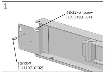
Before installing the Electrical Distributor on a frame, install a #8-32x¼" Phillips panhead screw in the upper tapped hole on the distributor base end to be installed next to the Vertical Distributor. Fasten a hex standoff to the end of the screw and tighten with a ¼" wrench and #2 Phillips screwdriver.
