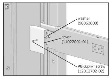
Insert a #8-32x¼" Phillips flathead screw through the countersunk hole in the cover, then a nylon washer, and align it with the tapped hole in the hex standoff. Tighten screw with a #2 Phillips screwdriver.
