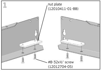
Before installing Data Distributors on the frames, the guide mounting screws must be assembled to the corner end of each distributor base. Align a nut plate, countersunk side down, with the holes in the base and insert two #8-32x½" Phillips flathead screws from the bottom of the distributor. Tighten screws with a #2 Phillips screwdriver.
