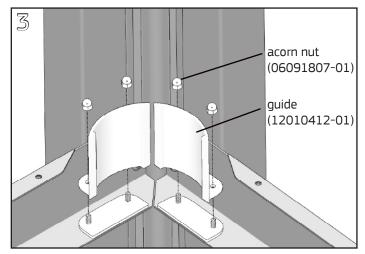
Align the holes in the bottom of each guide with the screws assembled in step 1. Fasten with a #8-32 acorn nut on each screw. Tighten nuts with a %6" nutdriver.
