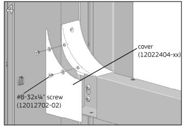
After routing data cables, attach the cover by fastening it to the entry guide with the two #8-32x¼" Phillips flathead screws.
