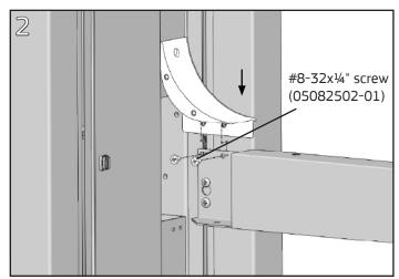
Slide the support bracket behind the Data Distributor base, aligning the holes in the support bracket with the two holes in the corner of the base. Fasten with two #8-32x¼" Phillips pan head screws using a #2 Phillips screwdriver.
