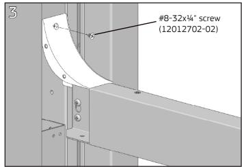
Attach the entry guide to the Vertical Distributor slider with a #8-32x¼" Phillips flathead screw.
