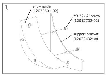
Assemble the entry guide to the support bracket with two #8-32x¼" Phillips flathead screws using a #2 Phillips screwdriver. The counterbored hole in the entry guide should be near the top portion of the support bracket.
