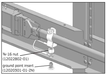
Place the ground point insert in the knockout hole with the flange on the outside of the distributor bottom. Place the ground wire ring terminal over the threads and fasten with a %-16 hex nut. Tighten with a %-1 wrench on the ground point insert flats, and a %-6" wrench on the nut. Test ESD ground path.
