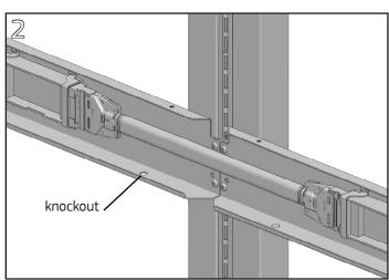
Punch out one of the knockouts in the bottom wall of the Electrical Distributor, located 4.5" from the left or right end.
