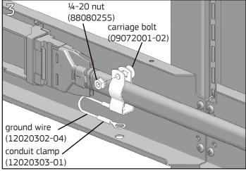
Slide the conduit clamp up over Electrical Distributor Jumper Cable, orienting the ground wire down. Insert a ¼"-20x¾" carriage bolt through the square hole in the clamp. Fasten with a ¼-20 hex nut and tighten using a ¾6" wrench/nutdriver so the conduit clamp makes contact with, but does not crush, the jumper conduit.
