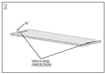
Remove the protective backing from the piece of Velcro loop. Press it firmly ¼" from each edge of the shelf.
