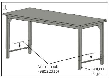
Remove the protective backing from the piece of Velcro hook. Press it firmly onto the shelf support bars.
