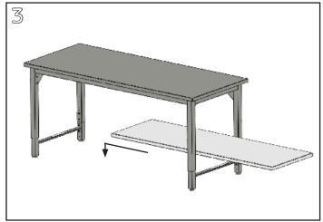
Position the shelf so the Velcro hook on the shelf support bars is in line with the Velcro loop on the shelf. Rest the shelf flat on the support bars.
