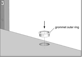
Disassemble the grommet and align the outer ring with the hole in the surface. Gently push the outer ring into the hole. If necessary, use a rubber mallet to tap the grommet ring down until the flange sits flush on the surface.
