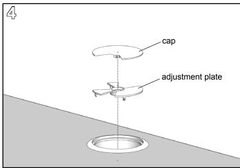
Reassemble grommet adjustment plate and cap in the outer ring.
