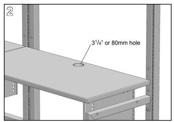
Using a power drill with a clutch and hole saw as described above, drill a hole through the surface at the marked location.
