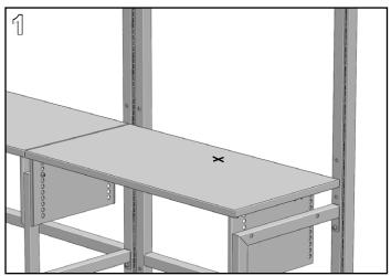
Ensure that surface is securely fastened to supports or otherwise secured in a work holding device. Mark the desired grommet center point on the top of the surface.
