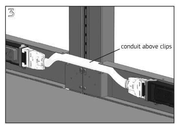
Connect jumper cable to the junction block at the other end and route the conduit above the hanger clips supporting the Electrical Distributors. Install covers per appropriate installation instructions.
