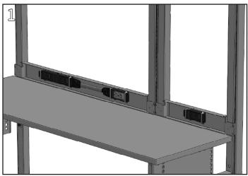
Install Electrical Distributor bases per appropriate installation instructions. Do not assemble covers.
