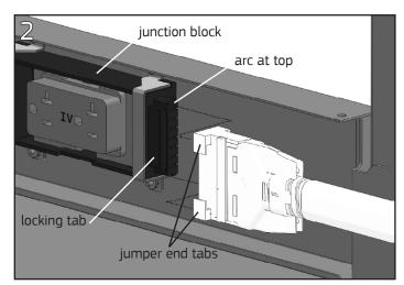
Align the end of the jumper cable with the end of one of the electrical junction blocks and slide onto the locking tab of the junction block until it clicks behind the jumper end tabs. Note the jumper is not symmetrical top to bottom, the arc-shaped opening on the jumper end must be oriented at the top.
