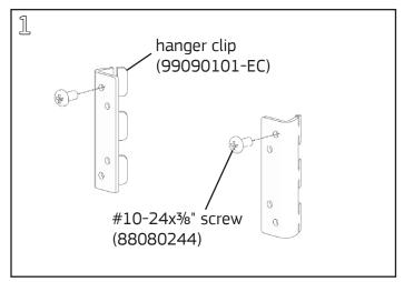
Install a #10-24x3%" Phillips pan head screw into the top tapped hole of each hanger clip. Leave a 1/8" gap between the head of the screw and face of the clip.
