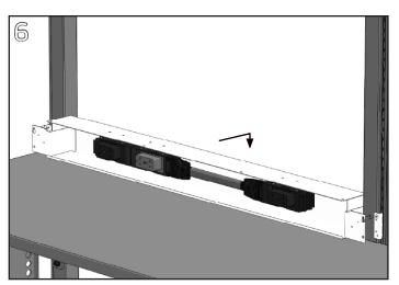
Align the bottoms of the keyslots in the Electrical Distributor base with the heads of the #10-24 screws in the hanger clips from step 2. Slide the distributor down over the screws to engage.
