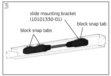
Remove the junction block assembly from the Electrical Distributor base by depressing the back plastic snap tabs at the top of the blocks and sliding the junction block forward until it clears the slide mounting brackets.
