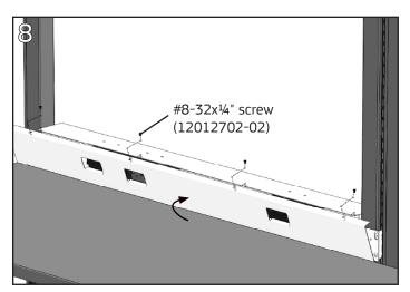
Holding the Electrical Distributor cover at a slight angle, align the opening with the duplex receptacle and rotate until the cover flange is on top of the base. Align all countersunk holes in the cover with the holes in the base. Install a #8-32x¼" Phillips flathead screw in each countersunk hole and fully tighten with a #2 Phillips screwdriver.
