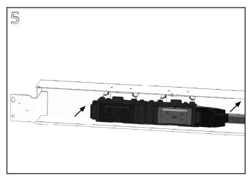
Align the tops of the junction blocks with the slide mounting brackets and slide the junction block assembly back into the Electrical Distributor base until it clicks into place.
