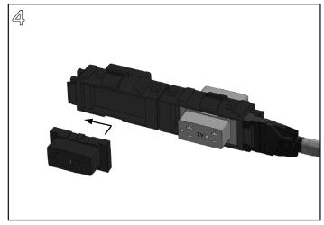
Install the Duplex Receptacles by inserting the receptacle into the junction block and sliding it to either the left or right until it clicks into place. Note the rear receptacle can only be installed/reconfigured when the junction block assembly is fully removed from the Electical Distributor base.
