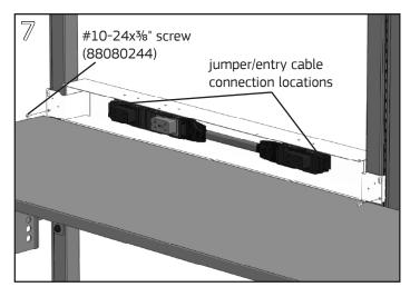
Install an additional #10-24x36" Phillips pan head screw in the hole below the keyslot in each hanger clip. Fully tighten all hanger clip screws with a #2 Phillips screwdriver. Install required jumper/entry cables at the connection locations per additional instructions before proceeding to step 8.
