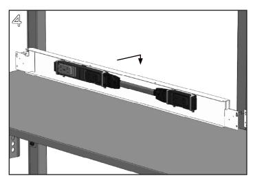
Align the bottom of the keyslots in the Electrical Distributor base with the heads of the #10-24 screws in the hanger clips from step 2. Slide the distributor down over the screws to engage.
