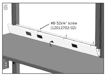
Holding the Electrical Distributor cover at a slight angle, align the opening with a duplex receptacle and rotate until the cover flange is on top of the base. Align all countersunk holes in the cover with the holes in the base. Install a #8-32x¼" Phillips flathead screw in each countersunk hole and fully tighten with a #2 Phillips screwdriver.
