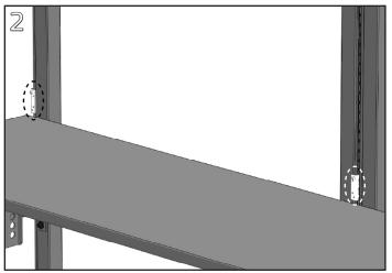
Install a hanger clip on the left and right side of the frame at the same height with the screws at the top of each clip.
