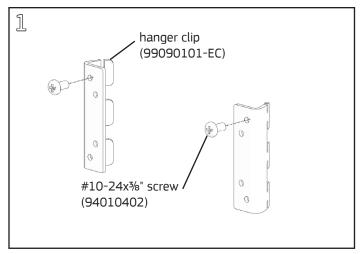
Install a #10-24x3%" Phillips pan head screw into the top tapped hole of two hanger clips. Leave a 1/8" gap between the head of the screw and face of the clip.
