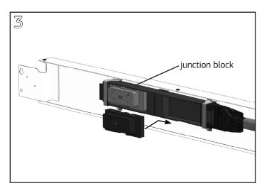
Install the Duplex Receptacles by inserting the receptacle into the junction block and sliding it to either the left or right until it clicks into place.
