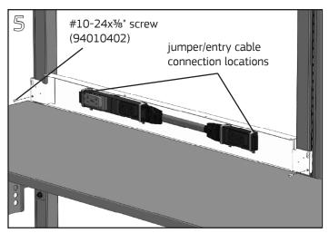
Install an additional #10-24x3/6" Phillips pan head screw in the hole below the keyslot in each hanger clip. Fully tighten all hanger clip screws with a #2 Phillips screwdriver. Install required jumper/entry cables at the connection locations per additional instructions before proceeding to step 6.
