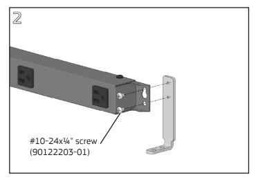
Fasten plug strip to bracket with (2) #10-24x¼" Phillips pan head screws using a **#2 Phillips screwdriver**. Repeat on the opposite end of the plug strip.
