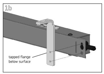
Align the keyslot hole and lower hole on one end of the Electric Plug Strip with the two tapped holes in one of the Surface Accessory Brackets. The plug strip can be mounted on the front or back of the bracket and the bracket can be mounted with the tapped flange above or below the surface.
