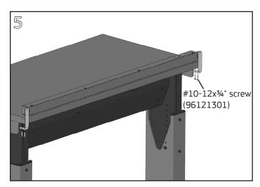
Reposition plug strip and fasten each bracket to the underside of the work surface with (2) #10-12x<sup>3</sup>/<sub>4</sub>" Phillips pan head screws using a #2 screwdriver/drill with bit.
