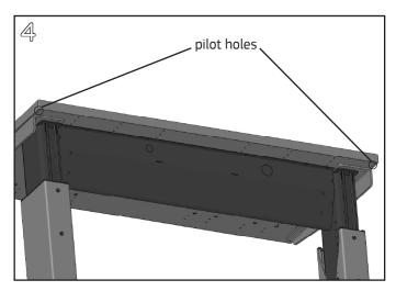
Using a drill bit and cordless drill, drill a pilot hole in the surface in the marked locations. Do not drill holes deeper than ¾" to avoid puncturing the top of the work surface.
