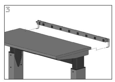
Install the work surface according to surface support instructions. Position the plug strip as desired with the flange and two thru holes held tight against the underside of the surface. Mark the hole locations on the underside of the surface for each bracket.
