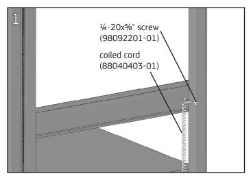
Install the component to be grounded according to instructions. Attach one end of the coiled ground cord to the threaded insert in the bottom or back of the component using a ¼-20x%" Phillips pan head screw and a #2 Phillips screwdriver.
