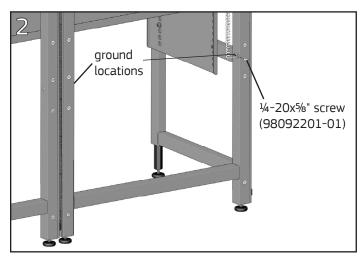
Determine grounding location. If grounding to the frame, attach the other end of the coiled cord to one of the threaded inserts on the inside vertical tube of the frame using a ¼-20x%" Phillips pan head screw. If grounding to a Common Point Ground plate, use the ¼-20x%" screw provided with ground plate to attach the coil cord to the plate.
