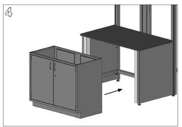
Install work surface according to Lab Leg installation instructions. Slide Base Cabinet into position.
