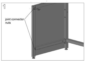
Install Lab Leg Panel according to its installation instructions. Leave the two joint connector nuts along the front tube of the Lab Leg loose leaving approximately an 1/8" gap between the leg and nut.
