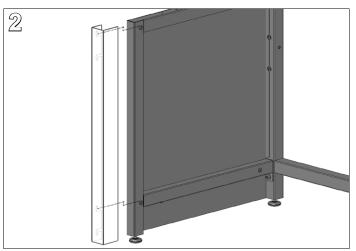
With the slotted side of the Lab Leg Filler against the leg, slide the filler onto the leg nuts at the top and second from bottom dog leg slots. Tighten the Lab Leg joint connector nut fully with a 5mm Allen Wrench.
