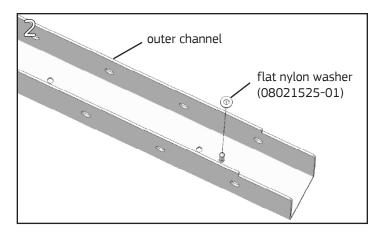
Place a nylon washer on the PEM stud on the outer channel of each reinforcement bar.
