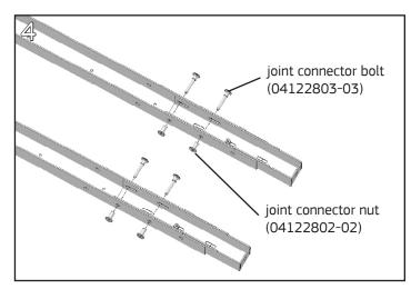
Insert a joint connector bolt and nut through the outer channel holes and through the appropriate inner channel slot location. Do not fully tighten.
