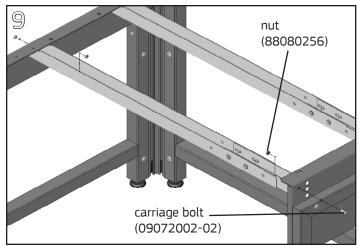
Repeat step 8 with the other Reinforcement Bar assembly at the front position per the diagrams in step 7. Note: Depending on the front bar position, it may be necessary to insert the carriage bolt into the square hole in the Frame-mount Surface Support before fully tightening this bracket to the clip.
