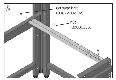
Insert one of the Reinforcement Bar assemblies in the rear position between the surface supports, bringing the bar up from below to clear the bracket flanges. Insert ¼-20x¾" carriage bolt into the square holes in the sides of the Frame-mount Surface Supports/B Supports and fasten each with a nut. Tighten the nuts with a ¾16" Nut Driver.
