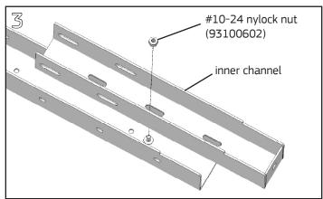
Position Reinforcement Bar inner channels on the inside of the outer channels as indicated in step 1. The PEM studs will align with one of the slots in the bottom of the inner channel. Loosely fasten with a #10-24 nylock nut.
