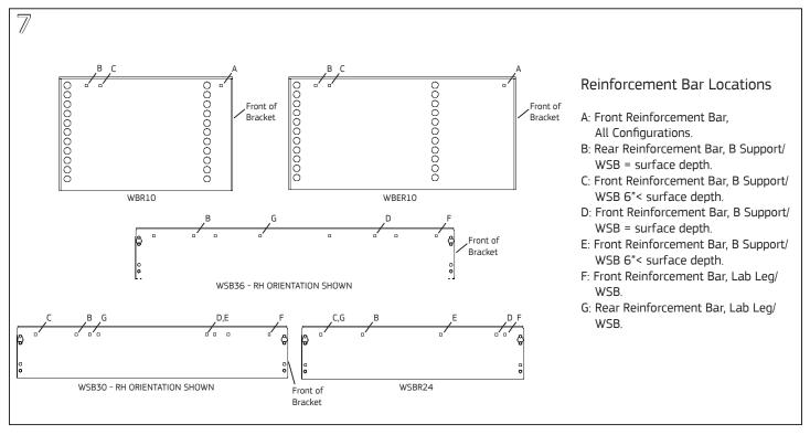
Install Frame-mount Surface Supports (WSB) and/or B Supports (WB, WBE) per product installation instructions. Based on the diagrams above, identify the front and rear Reinforcement Bar locations.
