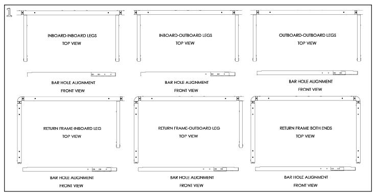
Determine leg configuration at location where Reinforcement Bars are to be installed. Note the required position of the slots in the inner channel relative to the holes in the outer channel shown in the corresponding "Bar Hole Alignment" views (the return frame-inboard leg configuration is shown throughout the remaining steps of these instructions).
