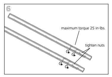
Tighten connections at the bar joints to a maximum torque of 25 in-lbs. using a **Torque Wrench** with **5mm Bit**. Then fully tighten the nut on the PEM stud in each of the channels with a **3/8**" **Nut Driver**
