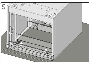
Push the pedestal back until the attachment screws lock into the two spring clips located at the front of the pedestal.
