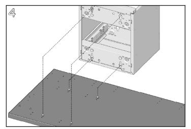
With the pedestal upside down, position the large keyslot openings in the pedestal top over the attachment screws.
