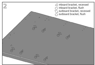
Determine left-right mounting position for pedestal based on location of the surface supporting bracket. The pedestal can also be positioned flush or recessed relative to the front edge of the surface.
