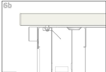
Return surface to an upright position and install as required.
