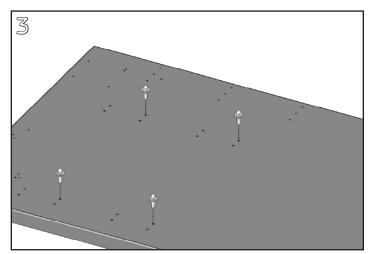
Install the attachment screws into the four pilot holes with a 3/8" nut driver.
