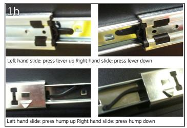
6" box drawers (bottom row) have disconnect levers actuated by pressing the hump area. 12" drawers (top row) have a shorter straight lever. In both cases, the lever needs to be pushed up on the left-hand slide and down on the right-hand slide while pulling out on the drawer.
