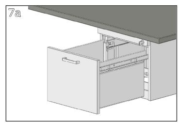
Use care to reinstall the drawer. Damage may occur to the slides, particularly the ball bearings, if the drawer is not installed properly. To properly reinstall the drawer, slide the ball bearing cartridges in the middle slide members of the pedestal to the front of each slide
