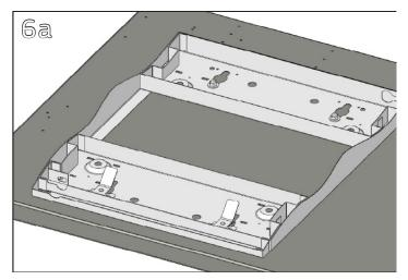
Assure that all four screws are securely engaged with the top of the pedestal as shown.
