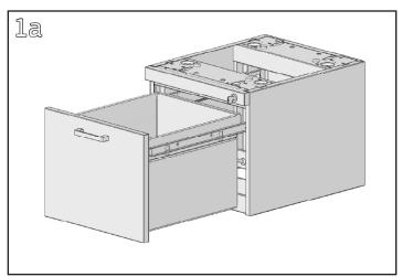
Remove the drawers from the pedestal by fully opening the drawers and then disconnecting the slide members.
