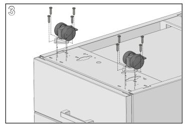
Align the locking swivel casters with the diagonal spaced holes at the front of the pedestal. Install (4) screws in the caster plate of each caster using a #2 Phillips Screwdriver.
