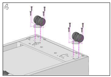
Repeat step #3 with the non-locking swivel casters at the rear of the pedestal.
