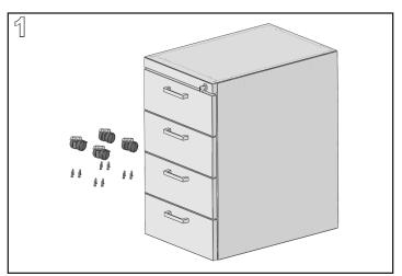
Locate the casters and attachment screws in one of the drawers of the pedestal. Lock or remove the drawers to ensure that they are not damaged during caster installation.
