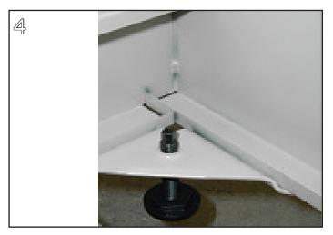
Adjust the four levelers to accommodate uneven or sloped floors with a ¼" wrench or socket. Replace the cabinet bottom and shelves.
