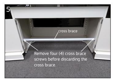
Each LUCA (door-to-floor) base cabinet is shipped with a cross brace support that must be removed after the cabinet is installed and leveled. Remove and discard the screws at each end of the cross brace. Then, remove and discard the cross brace.
