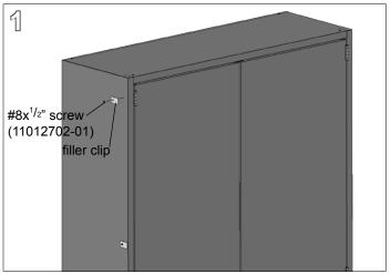
Using a **cordless drill with magnetic socket driver** and #8x1/2" hex washer head screws, install four filler clips vertically on the wall side face of the case with a setback of approximately 1-3/4". The floor case is not predrilled for the clips.
