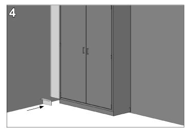
If desired, the top flange of the toe space filler can be cut down to align with the floor case base. The toes space filler is not provided with a means of attachment. It is suggested that the filler be placed in the space between the case and wall, and adhered using either epoxy glue, pop rivets, or other fastening method.
