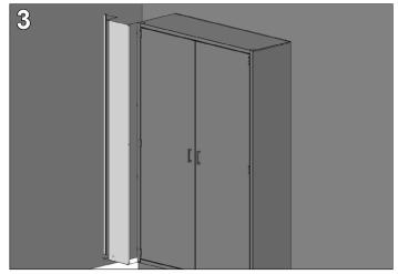
Slide the long flange of the filler into the slip joint and the short flange of the filler into the filler clips on the floor case. The filler is held in place with a friction fit only, no additional fasteners are needed.
