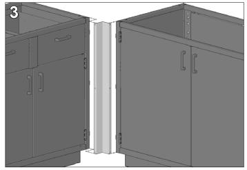
Slide the corner filler into the filler clips. The filler is held in place with a friction fit only, no additional fasteners are needed.
