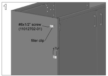
Using a cordless drill with magnetic socket driver and #8x1/2" hex washer head screws, install three filler clips vertically on the side face of the cabinet. The rear of the filler clip should have a setback of approximately 1-3/4". The cabinets are not predrilled for the clips.
