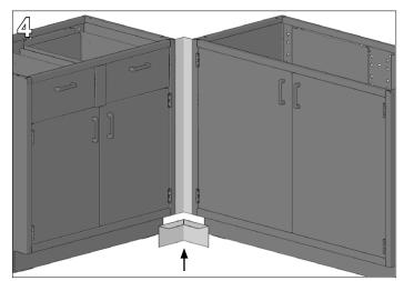
Bend the toe space filler. The toes space filler is not provided with a means of attachment. It is suggested that it be placed in the corner space between the cabinets and adhered using either epoxy glue, pop rivets, or other fastening method.
