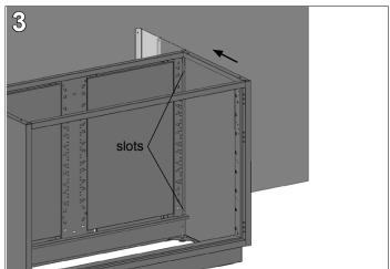
Align the side of the base cabinet with the side of the filler. Locate the horizontal slots near the top and bottom of the inside of the cabinet. Mark these locations on the short flange of the filler. Cabinet shelves and drawers may need to be removed to accomplish this.
