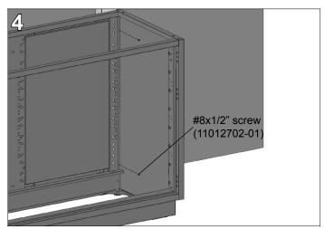
If desired, remove filler and predrill holes. From within the cabinet, using a **cordless drill with magnetic socket driver** and (2) #8x1/2" hex washer head screws, attach the back of the cabinet to the short flange of the filler.
