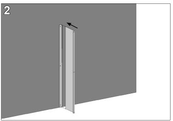
Slide the long flange of the filler into the slip joint. The filler is held in place with a friction fit only, no additional fasteners are needed.
