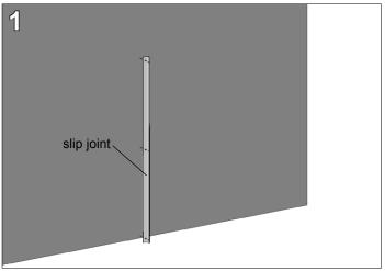
Fasten the slip joint to the wall as required. Attachment hardware for the slip joint is not included with the filler kit. Clearance holes in the slip joint are 1/4" diameter.
