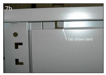
Locate the two factory-installed bent tabs in the upper flange of the cabinet back. Bend the tabs to a straight position, allowing the cabinet back to slide upward.
