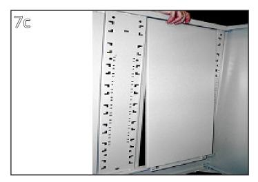
Slide the back panel upward, then push the bottom of the panel forward to remove it from the cabinet.
