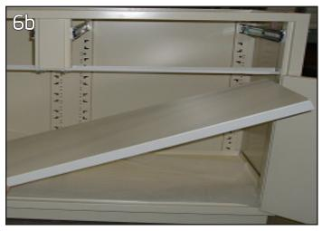
Tilt the shelf at an angle to place it in the cabinet, being careful not to scratch the inside of cabinet. At extreme shelf locations (top/bottom) it may help to install rear clips first, then rest the back of the shelf on the rear clips while holding up the front end of shelf. Then install the front clips.
