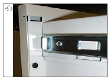
To reinstall drawers, pull the bearings all the way forward on the slides in the cabinet. Align the slides on the drawer within the slides in the cabinet. Push the drawer in with equal pressure on both sides. The black nylon lever on the slide attached to the drawer body will lock the drawer in place. Adjust drawers by loosening the screws in the lower inside corners of the drawer front. Grab draw front and slide it up/down. Tighten screws and check for fit. Repeat if necessary.
