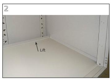
Install and level base cabinets and secure surfaces. Remove all shelves. Remove cabinet bottom panel by lifting up at the back edge, then tilt and remove.
