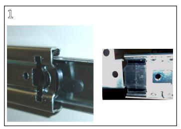
Remove drawers from the base cabinet: Locate the black nylon lever on each side. Simultaneously push the left lever and the right lever down while gently pulling the drawer out. (Certain levers may need to be pushed in). Pull the drawer body out of the slides. Note how the ball bearings engage in the grooves to lock the slide members together.
