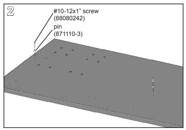
Flip the surface to be mounted to the bracket(s) upside down. Locate the hole(s) dimensioned above and install a pin at each bracket location with a #10-12x1" screw using a **cordless drill** and **#2 Phillips bit**. Install necessary hardware on the other end of surface based on the mounting method.
