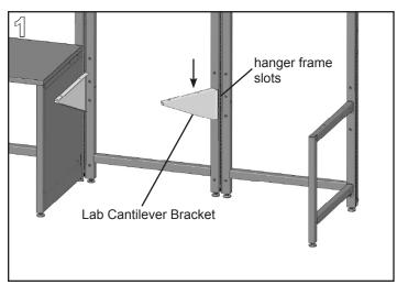
Rotate the Lab Cantilever Bracket at an angle inboard of the frame. Align with the hanger frame slots in the side of the frame at the appropriate height. Push the support down to securely seat in the slots. Surfaces 72" and wider require an additional support at the frame joint.
