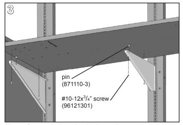
Flip surface and align pin with large diameter hole in the top face of the Lab Cantilever Bracket(s); rest the surface on the bracket. Install (2) #10-12x³/₄" Phillips screws through each bracket into the surface, one in front of the pin and one near the back of the surface. Tighten fully with a **cordless drill** and **#2 Phillips bit**.
