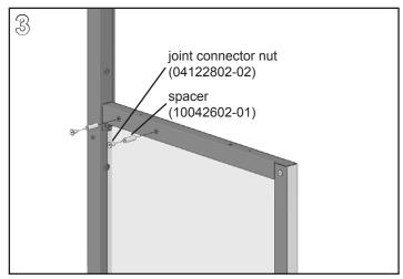
Insert a spacer into each of the holes in the top channel of the leg (24" deep has one hole, 30" and 36" depths have two holes). Fasten with a joint connector nut through each spacer/leg/bracket assembly. Tighten all nuts securely.
