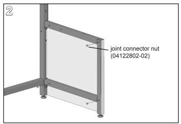
Loosely fasten the panel to the leg with a joint connector nut through the bottom leg holes and the top front hole in the leg.
