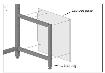
Align the PEM studs in the Lab Leg Panel with the holes in the side of the Lab Leg.
