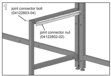
Orient the bracket as needed with the pin hole located near the front of the lab leg (left-hand is shown). Align the front Lab Leg hole with the front hole in the side of the bracket and fasten loosely with the joint connector bolt and nut.
