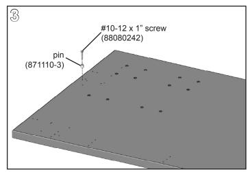
Flip the surface to be mounted to the bracket upside down. Locate the hole dimensioned above and install a pin with a #10-12x1-1" screw using a **cordless drill** and **#2 Phillips bit**. Install necessary hardware on the other end of surface based on the mounting method.
