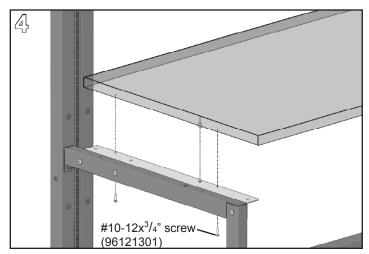
Flip surface and align pin with large diameter hole in the top face of the Adjacent Bracket; rest the surface on the bracket. Install (2)  $\#10-12x^3/_4$ " Phillips screws through the bracket into the surface, one in front of the pin and one near the back of the surface. Tighten fully with a **cordless drill** and #2 **Phillips bit**.
