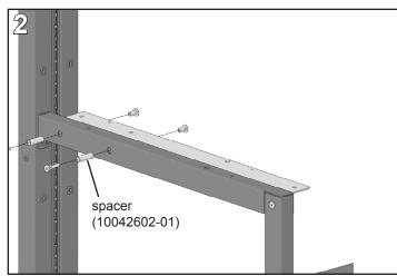
From the non-bracket side of the Lab Leg, insert a spacer into each of the holes in the top channel of the leg (24" deep will have one hole and 30" and 36" depths will have two holes). Fasten with a set of joint connector bolts and nuts through each spacer/leg/bracket assembly. Tighten all fasteners securely.
