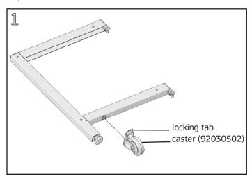
Leg with caster only - Locate the caster (shipped separately) and lock it by pressing the tab near the top of the wheel. Install the caster in the threaded hole in the bottom of the leg.
