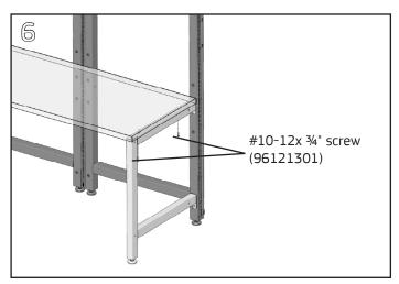
Install (2)  $\#10-12x^3/4$ " Phillips buttonhead screws through the top face of the Lab Leg into the surface, one in front of the pin and one near the back of the surface. Tighten fully with a **cordless drill** and a #2 **Phillips bit**.
