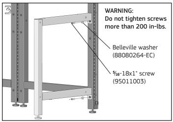
Fasten leg to frame/post with (2) Belleville washers, placed concave side against the tube, and (2) %6-18x1" cap screws using the ¼" Allen wrench/hex bit. For legs with a glide adjust the glide up or down until the leg is level.
