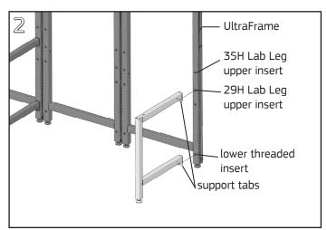
Align holes in the leg support tabs with the threaded inserts on the front or back face of an UltraFrame or Connector Post. The support tabs will mount flush against this vertical tube.
