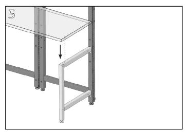
Flip surface and align pin with the large diameter hole in the top of the Lab Leg. Rest surface on Lab Leg.
