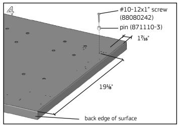
Surface installation (if applicable) - Flip surface upside down. Locate the hole dimensioned above and install a pin with a #10-12x1" screw using a **cordless drill and #2 Phillips bit**. Repeat on opposite end of surface if necessary.
