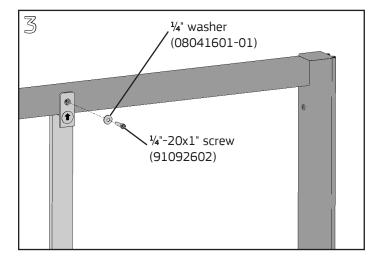
Fasten spine to frame at upper spine hole with (1) ¼" ID flat washer and (1) ¼-20x1" cap screw using a ¾6" Allen wrench/hex bit. Repeat at lower spine hole location. Rotate the Riser Frame toward the back of the ErgoStat so that the back of the Riser Frame blades rest on the bottom top support screws.
