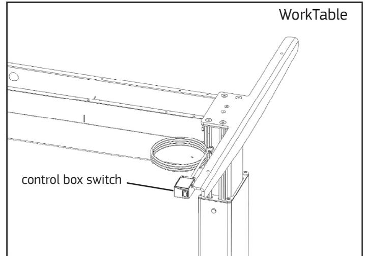
3. Plug unit into a 120-volt outlet. Adjust height of base by pressing the up/down switch on the control box.
