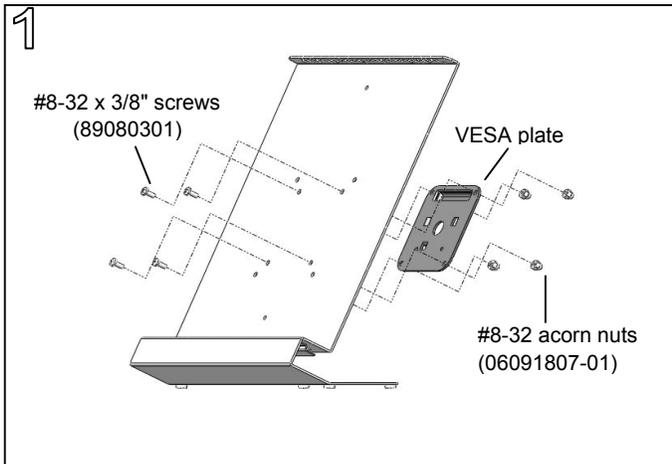
Install 75mm or 100mm VESA plate (from flat screen arm) to document holder using screws and acorn nuts provided. Tighten using a **5/16" open end wrench** and **#2 Phillips screwdriver**.
