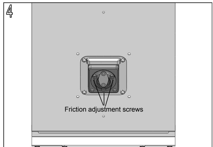
Friction on the ball joint can be modified by adjusting the (3) pre-installed socket head cap screws using a **4mm Allen wrench**.
