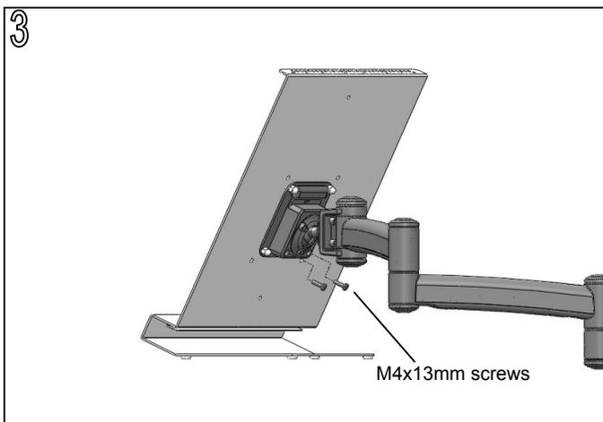
Secure VESA plate to ball joint by inserting (2) M4x13mm screws through ball joint into tapped holes in VESA plate. Tighten screws with **#2 Phillips screwdriver**.
