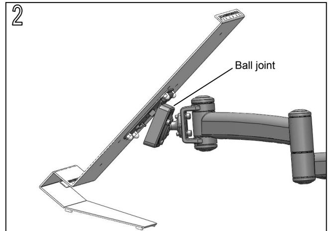
Mount VESA plate/document holder assembly to arm by sliding the large emboss on the VESA plate over the top flange of ball joint.
